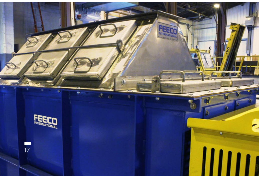
◀ Covered Pugmill Mixer with observation panels for use in animal feed production
