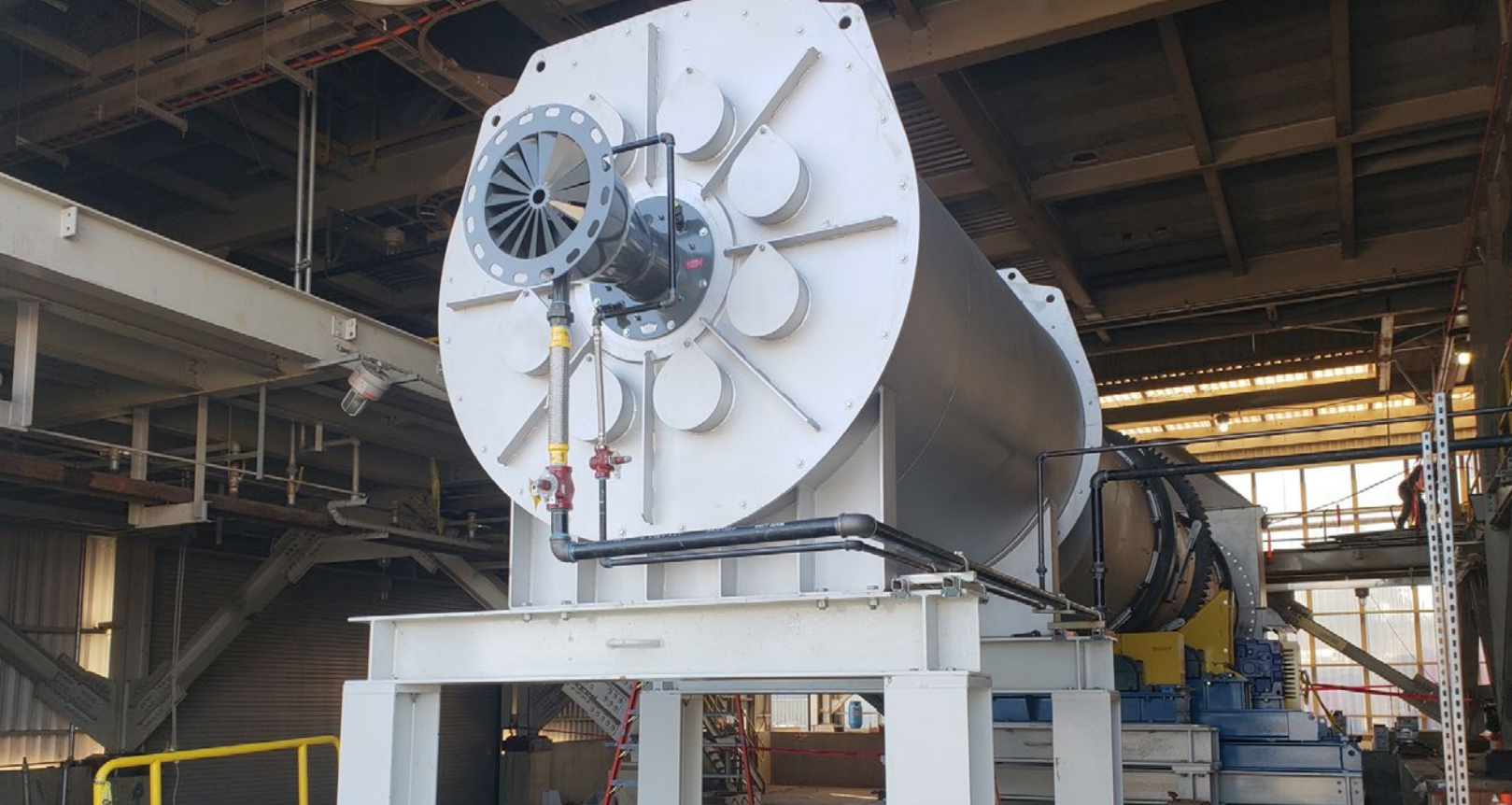
▲ Sand Dryer with Combustion Chamber
