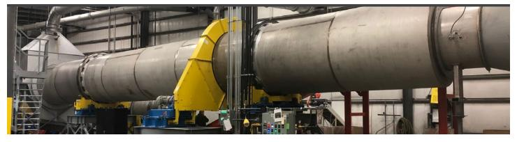
Direct rotary dryers rely on direct contact between the material and drying air. This direct contact, combined with the use of lifting flights, maximizes the heat transfer between the material and drying air, offering a highly efficient processing solution.
