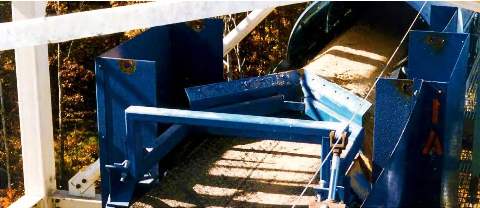
▲ Belt Plow in operation
