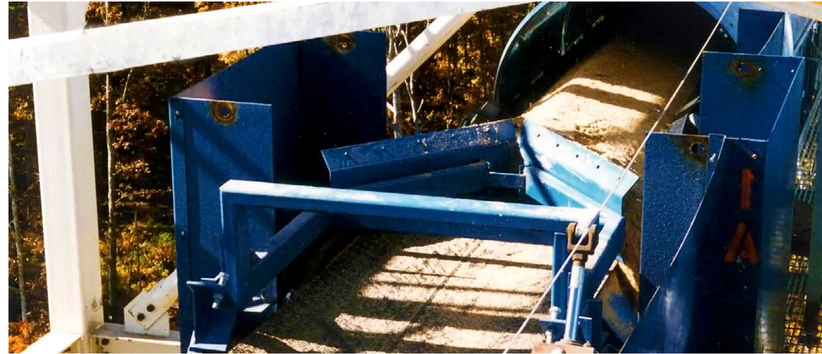
▲ Belt Plow in operation
