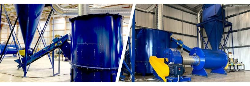
Fluid bed dryers offer a cost-effective alternative to rotary drying technology. With a smaller footprint and greater heat transfer efficiency, these industrial dryers are ideal for processing free-flowing, uniform solids such as fertilizers, specialty chemicals, biomass, and biosolids and are backed by the extensive expertise and process development capabilities that only FEECO International can offer.
