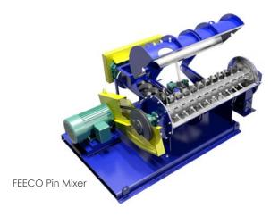
The <u>pin mixer</u> works as a primary feed conditioner to the gypsum pelletizing process, mixing the powdered gypsum with a liquid binder solution. The rotational motion of the pins imparts a spinning action to the gypsum mixture, reducing air and water volume between particles. The intense motion also results in densification many times that of a disc pelletizer. This step conditions gypsum, priming it for ideal pellet formation on the disc pelletizer.
