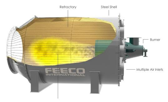
Burner Flame (totally contained inside chamber)
