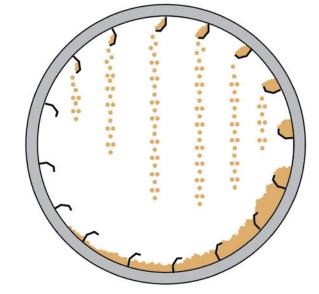
The diagram above illustrates how flights create the curtain in a rotary dryer to maximize heat transfer.
