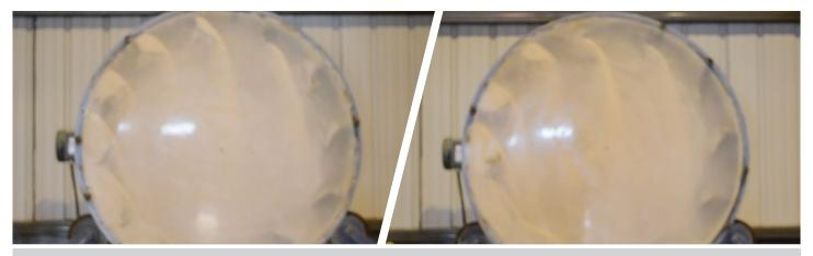
The pictures above show the same lifter configuration at two different rotational speeds. The picture on the left shows a good distribution of solids across the width of the unit. The gaps seen in the picture would be filled in by off-setting the lifters. In the picture on the right, the rotational speed is increased and the lifters empty later, giving a poorer distribution.
