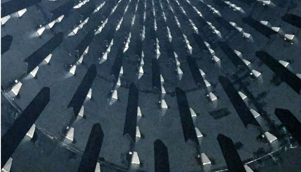
▲ Rotary Dryer Interior
