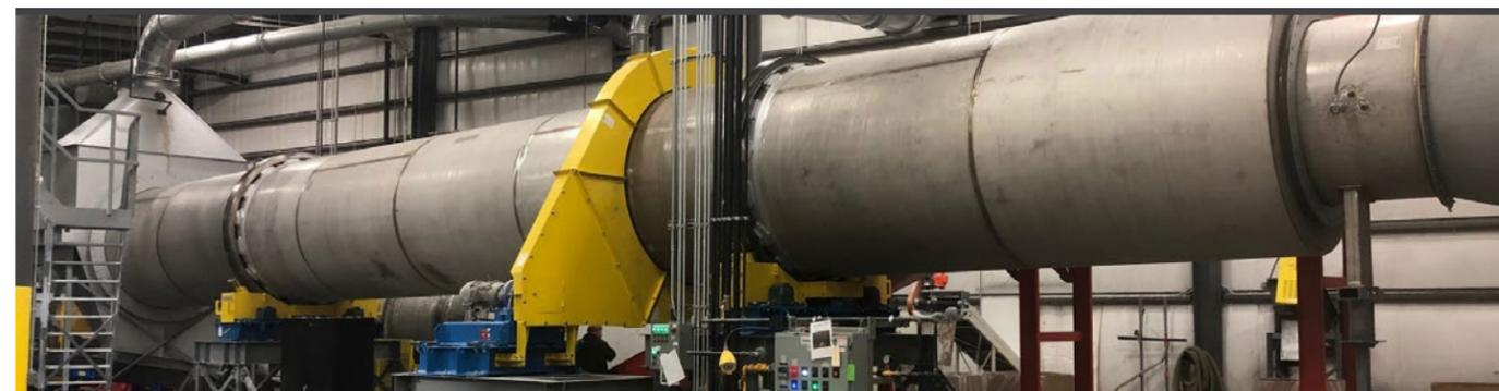
Direct [rotary dryers](#) rely on direct contact between the material and drying air. This direct contact, combined with the use of lifting flights, maximizes the heat transfer between the material and drying air, offering a highly efficient processing solution.
